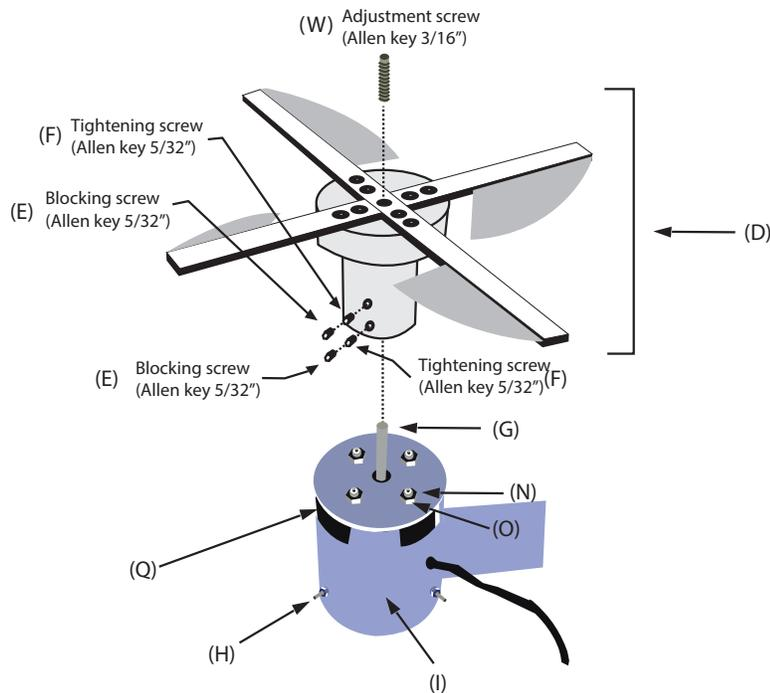
Remove the blade assembly (blade + tubular structure under it) (D). To achieve it, remove the 2 blocking screws (E) from the blade-hub and unscrew the 2 tightening screws (F). To remove the whole blade and blade-hub, raise it from the motor shaft.
