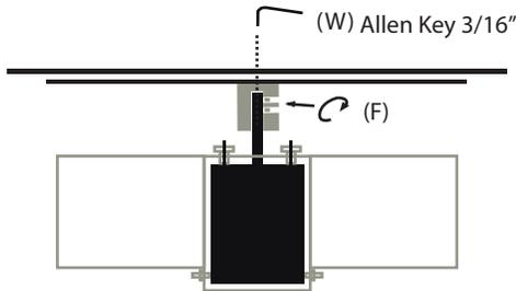
Once the blade is levelled out in relation to the grate, adjust the definitive height of the blade with the height adjustment screw (W). For security reason, a distance of at least 1/8 of an inch (3mm) between the grate and the blade is recommended. Tighten the tightening screw (F).
