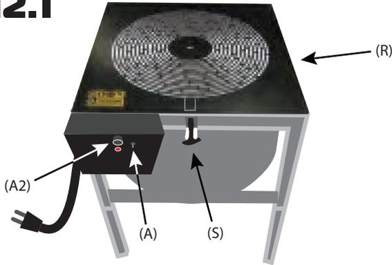
Close the lid of the machine (R) using the rubber fasteners (S), raise the speed a bit using the speed adjustment knob on the control panel (A2) and check if the electricity arrives to the motor (if the motor shaft is turning). If everything works correctly, turn OFF the machine with the On-Off switch (A) and unplug the machine from the electrical outlet. If the motor is not turning, contact us.
