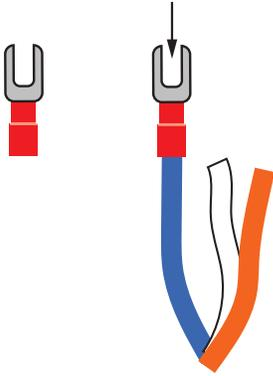
Install the connectors provided with the motor at the end of each wires coming out of the replacement motor. Take some pliers to make sure the connectors are fixed at the end of each wire.
