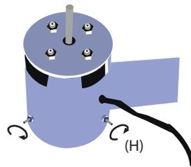
Once the optimal height is achieved, reinstall the blocking screw (E) to fix the blade (C) and the blade-hub (D) (in one piece) over the motor shaft. Tighten smoothly the motor-hub bolts (H) until they touch the surface. **(Beware! Too much pressure on the motor can damage it)**. Tighten the motor-hub nuts. Test again. If everything is OK, you can use the machine.
