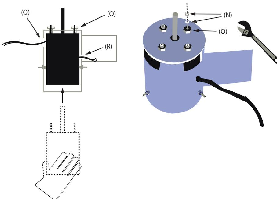
Install the new motor placing the wires on the opening situated on the side of the motor-hub (Q). Place the motor rods inside the drilled bolts (O) (like the old motor). To fix the motor, push it up to the maximum in the motor-hub structure and then reinstall by tightening the 4 nuts and 4 lock washers (N) on top of the motor-hub. Once again, do your best to make sure the bigger hexagonal bolts (O) do not move to avoid the blade recalibration.
