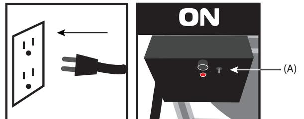
Plug the machine on the electrical on the electrical outlet and switch ON the machine with the ON-OFF switch (A).
