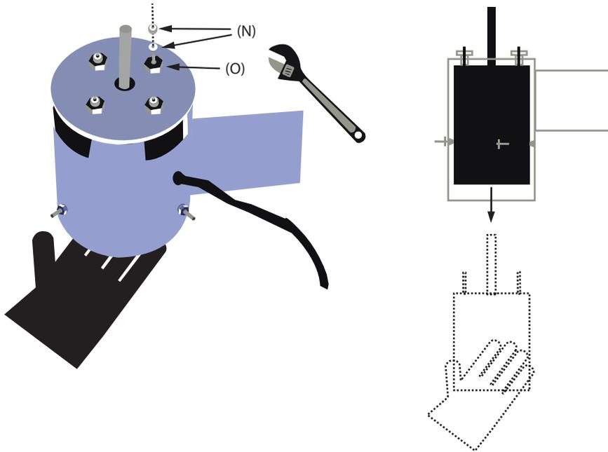
Hold the motor base (under the motor-hub) and remove the 4 nuts and 4 lock washers (N) that are fixed to the motor rods. Try not to move the bigger drilled hexagonal bolt (O), that way, you might avoid the recalibration of the blade later on. Remove the motor.
