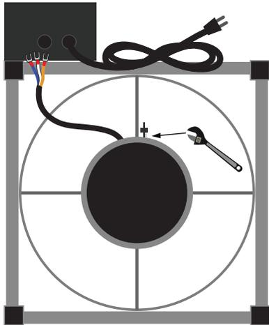
Pass the wires back inside the control panel (fig. 9.1) and install them according to the drive connection diagram (fig 9.2).
