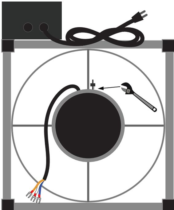
If you refer to the drive connection diagram on fig. 4.1, you have 6 wires at the bottom. The 4 wires starting from the left (1,2,3,4) need to be unscrewed (you don't need to remove the screw completely, just enough to be able to remove the wire) and pulled out from the control box. You then have to pull those same wires into the inside frame like on figure 4.2.
