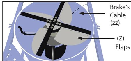
**YES** Change manually the angle of the flaps if necessary
