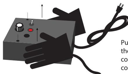
Put the machine on it's back (fig.3.1), remove the 2 screws from the front panel of the control box and remove the front plate of the control box like on fig. 3.2.
