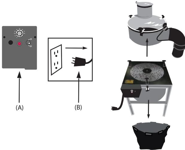
Turn off the machine with the ON-OFF switch (A) on the control panel and unplug the power cord (B) from the electrical outlet. Remove the bag using the Velcro strips on top of it and remove the circular aluminium & plastic structure using the rubber fasteners.
