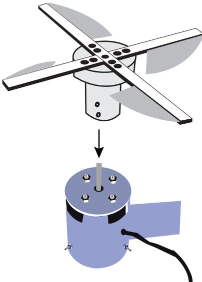
Reinstall the blade assembly on the machine in one piece without tightening the tightening screw.
