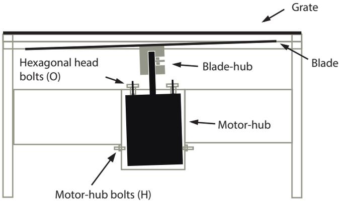
Check if the blade is at equal distance to the grate from each of its extremities (Y1 & Y2).
