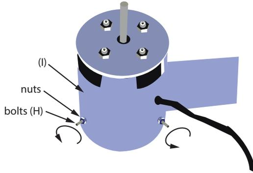
Unscrew the 3 nuts and then the 3 bolts (H) on the side of the structure which hold the motor (later referred as the motor-hub) (l).
