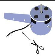
Cut the actual electrical wiring connections with a scissor.
