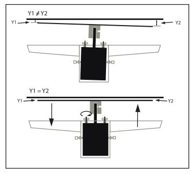
Check if the blade is at equal distance to the grate from each of its extremities (Y1 & Y2).
