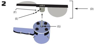
Remove the blade assembly (blade + tubular structure under it). This structure is called the blade-hub (D). To achieve it, remove the blocking screw (E) from the blade-hub and unscrew the tightening screw (F). To remove the whole blade and blade-hub, raise it from the motor shaft (G).
