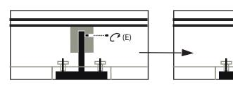
Once the optimal height is achieved, reinstall the blocking screw (E) to fix the blade (C) and the blade-hub (D) (in one piece) over the motor shaft. Test again. If everything is OK, you can use the machine.
