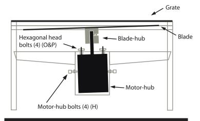
**TO RAISE ONE SIDE OF THE BLADE,** TURN CLOCKWISE THE BOLT **ON THE OPPOSITE SIDE** OF THE SIDE TO BE RAISED.
