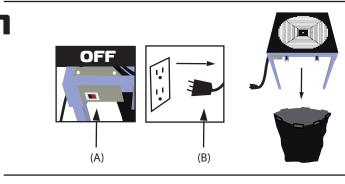
Turn OFF the machine with the ON-OFF switch (A) and unplug the power cord (B) from the electrical outlet. Remove the bag using the Velcro strips on top of it.
