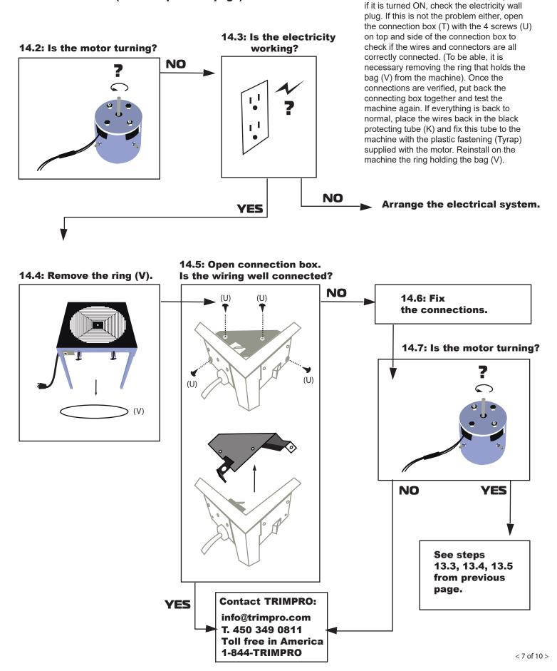
If the machine does not work properly even
